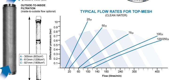
The heart of the Top-Mesh tubular element is a spiral wire structure of stainless steel which gives the support necessary to cope with higher operating/differential pressures and liquid viscosities.
